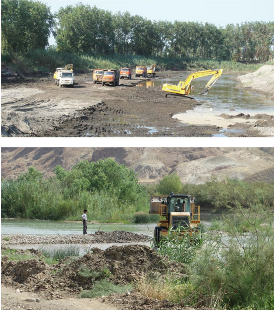
Fig. 17.3 Harvesting sand from riverbed. Above: in Mazandaran Province's rivers, in the southern Caspian Sea basin (photo from www.pana.ir ), below: Ilam Province, in the Tigris River basin
