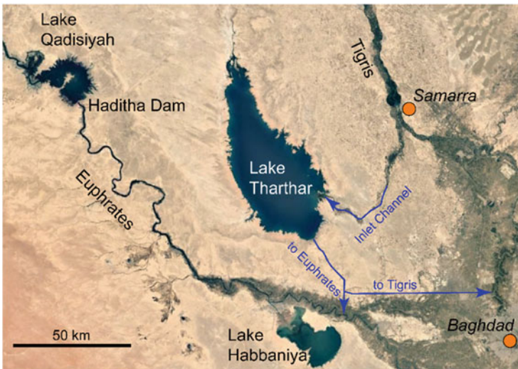
Fig. 13.6 Location map of the Lake Tharthar System (aerial photo from Google Earth). Inlet channel and outlet channels are highlighted
