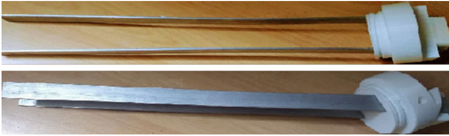
Fig. 2 Two stainless steel electrodes 51 cm long and 1-inch width each with thickness 3 mm
