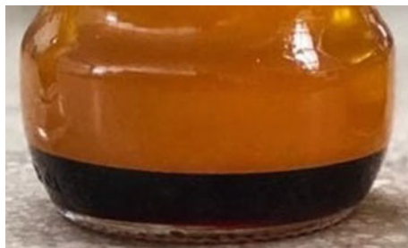
Fig. 3 Interface line between Biodiesel and Glycerol when the mixture finishes settling
