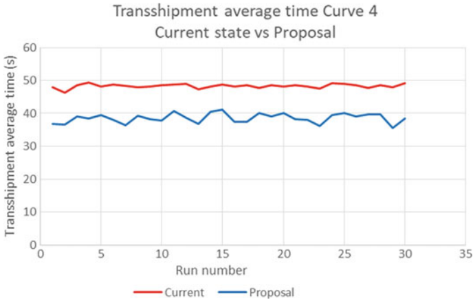
Fig. 7 Comparative chart of current delays versus delays generated with the proposal for transshipment 4
