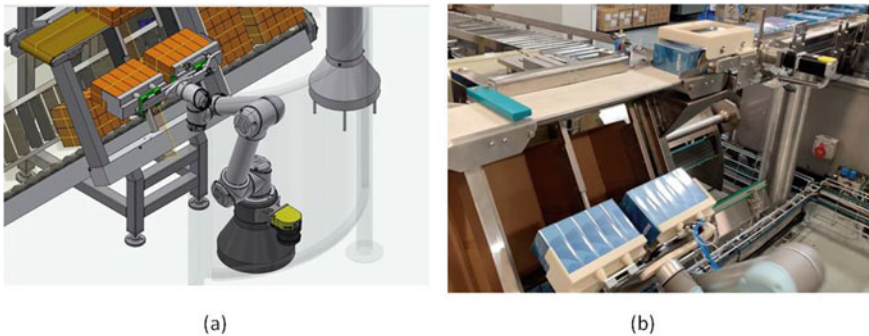
Fig. 4 Final implementation: a deployment 3D simulation in the factory layout and b the robot finally installed on the production line
