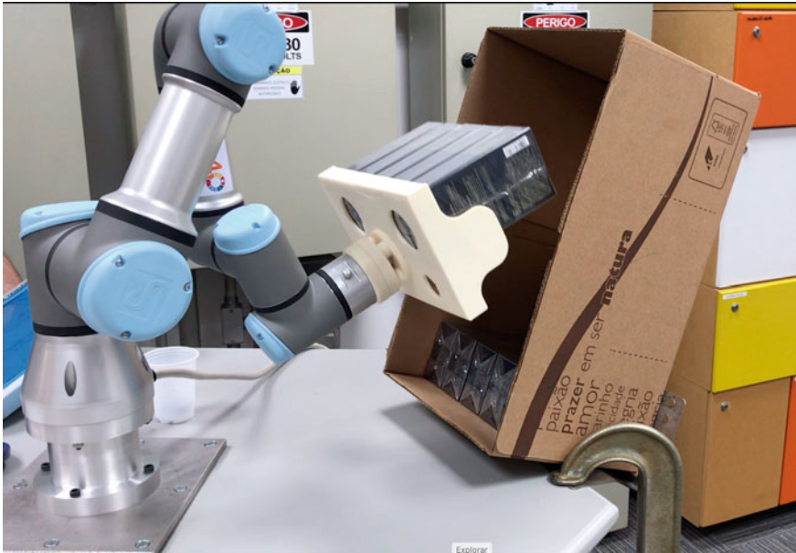
Fig. 2 Testing the gravity sliding of a set of product units to the shipping box
