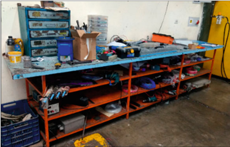
Fig. 5 Mechanical and electrical area prior to using 5 S
