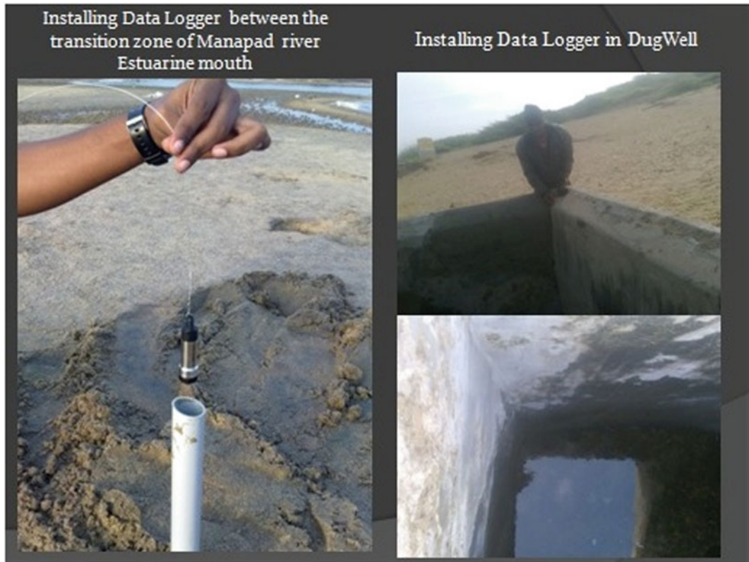
Fig. 14.9 Tidal level and groundwater level measurements
