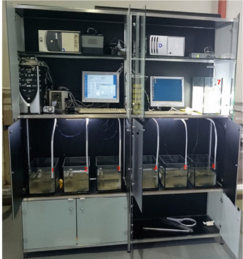
Fig. 10.2 A picture of a System for Industrial Biological Water Quality Monitoring (BioArgus-W) set up at one of water intakes of St. Petersburg. The lightproof doors (usually closed) are opened for demonstration. 1–6—numbering of flowing aquariums with crayfish; 7—a flowing aquarium with a few fishes
