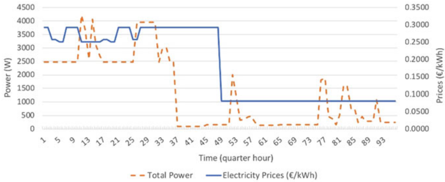
Fig. 1.1 Best solution obtained by PSO for the Free BL I model with adjacent mutation in the price labels vectors
