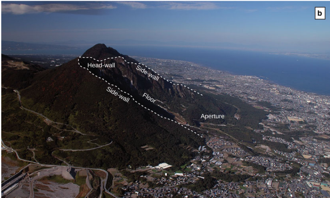
Fig. 2 Descriptive elements and dimensions for a volcanic landslide scar. a Cross-sections and plan view with the main descriptive terms and geometrical parameters defined in Table 2. b Mayuyama landslide scar, Japan
