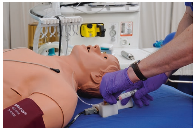
Fig. 12.5 CAE HPS® Human Patient Simulator uses bar code technology for its drug recognition system that allows the system to identify the concentration and dose of the drug administered. (Photo courtesy of © 2016 CAE Healthcare. All rights reserved)
