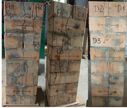
Fig. 4. Crack patterns after damaging by axial loading
