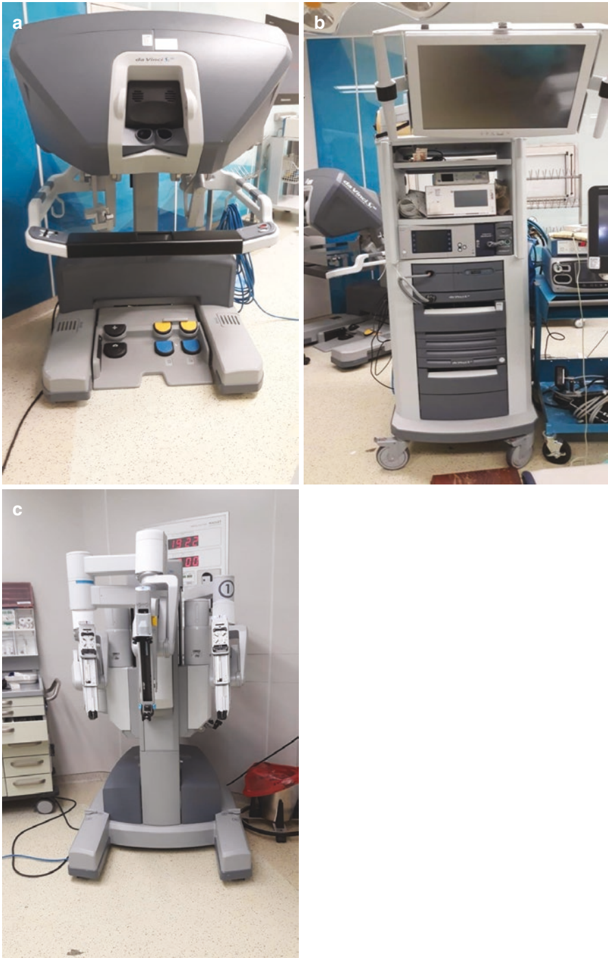
Fig. 17.1 da Vinci Robotic System (a) the console, (b) video processor, (c) robotic arms
