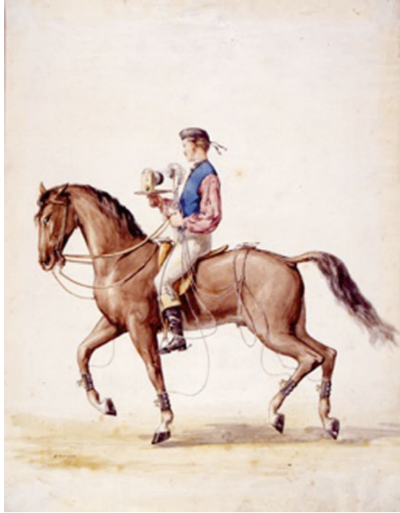
Fig. 4.1 A artistic representation from Marey's graphical method. Horse and Rider with inscribing apparatus: Rubber balls are attached under the horse's shoes (right part) and connected to a recording device by rubber tubing fastened along of its legs in order to portray the rhythm of the gaits of horse
