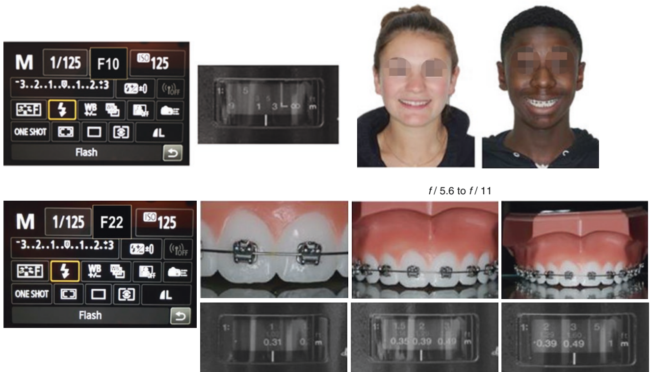
Fig. 2.13 Camera settings and magnification ratio for consistency of the views. These views may be taken either in manual (M) or aperture priority (Av) mode
