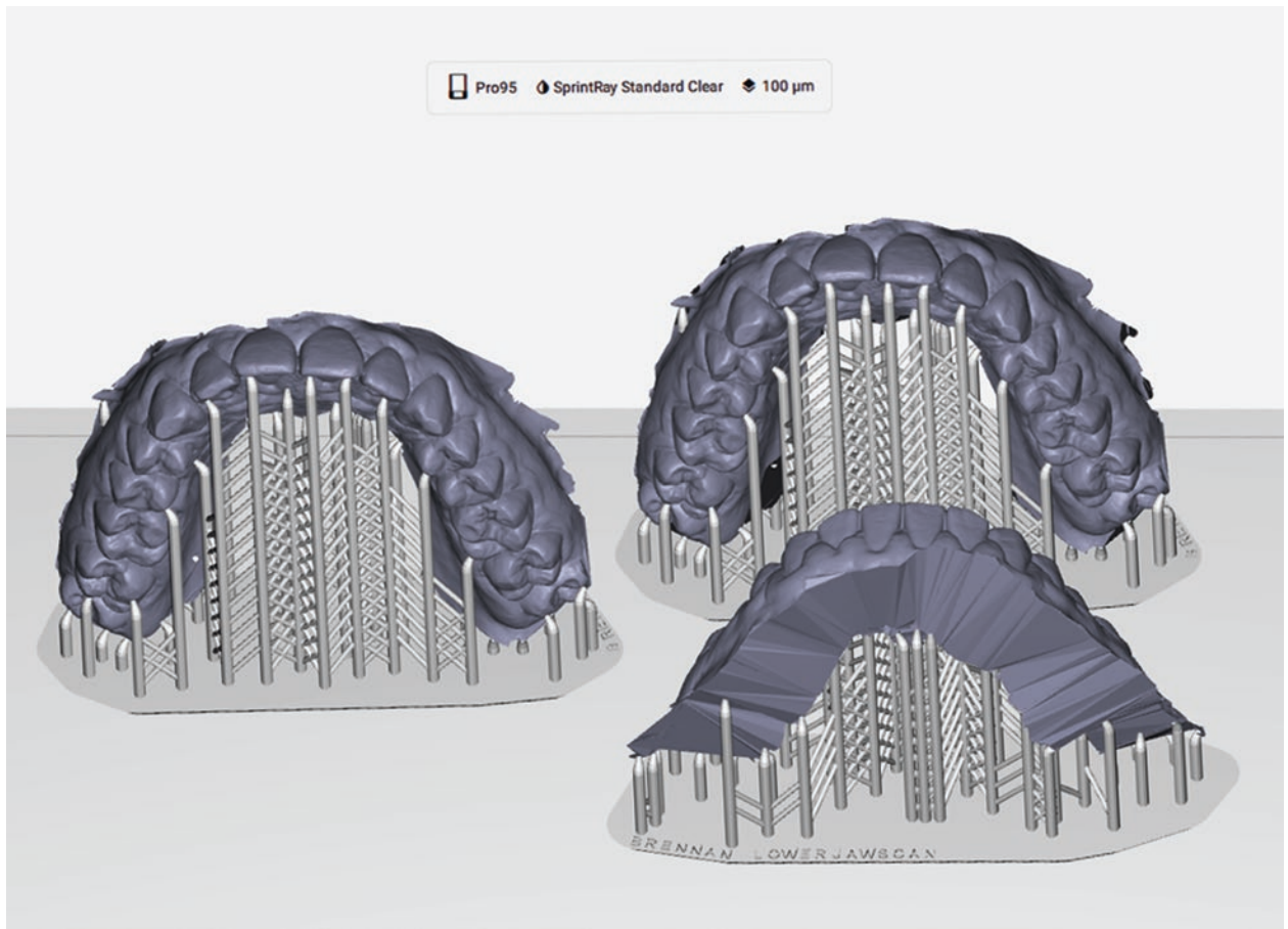
Fig. 6.23 The staged models in STL format to be ready for in-house 3D printing
