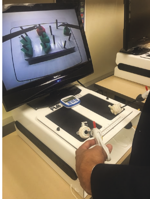
Fig. 28.1 Reality-based laparoscopic simulation. In this image, the operator is performing a task-based simulation commonly known as “peg transfer” using laparoscopic instruments to transfer objects from pegs on one side to pegs on the other side
