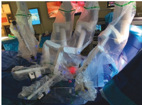
Fig. 21.3 Docked robot configuration: the robotic cart is brought in on the left side midway towards the end of the bed, the boom is deployed as far as possible and aligned with the target organ, and the arms are triangulated and docked. (© 2020 Intuitive Surgical, Inc. https://www.intuitive.com/en-us/about-us/press/press-resources )
