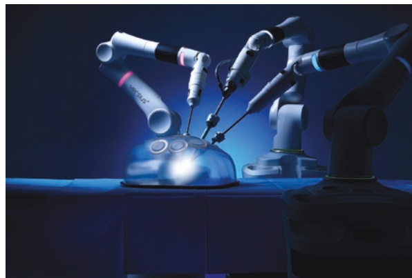
Fig. 27.2 Versius robotic system. (© 2020 CMR Surgical Ltd. Reproduced with permission)
