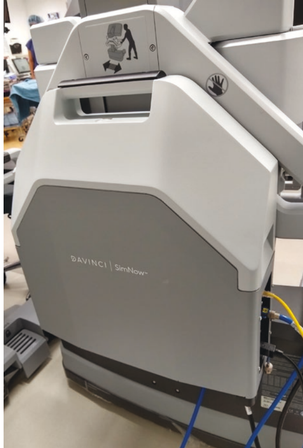
Fig. 28.4 A virtual-reality simulator designed for robot-assisted laparoscopic surgery simulation. This simulation system can be used for task-based and procedure-based simulation in robotic surgery
