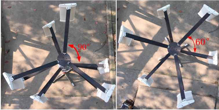
Fig. 13. Wind turbines at 90^\circ and 60^\circ double-layer installation angle
