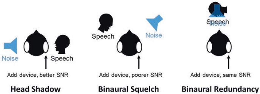
Fig. 13.3 Schematic representation of adding a second device to obtain benefits from the head shadow effect ( left ), binaural squelch ( center ), and binaural redundancy ( right ). Details regarding the potential benefits in each of these conditions are described in the text
