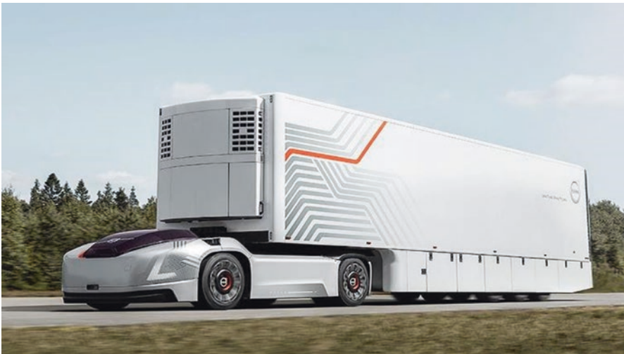
Fig. 3.4 Volvo's electric autonomous vehicle Vera. Note: Together with Vera Volvo also develops a system design for collaborative networks of autonomous vehicles that shows some similarities with the 4C concept
