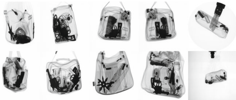
Fig. 2.8 Some X-ray images of a bag containing handguns, shuriken , and razor blades (group Baggage series B0048)
