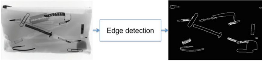
Fig. 4.15 Edge detection of an X-ray image of a pen case. The edges correspond the boundaries of the objects that are inside the pen case. [→ Example 4.11 📄]
