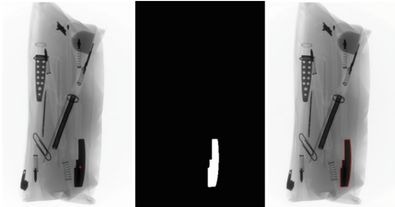
Fig. 4.29 Region growing in an X-ray image using a seed pixel in the object of interest. The region is well segmented as we can see in the binary image and in boundaries. [→ Example 4.9 🐍]
