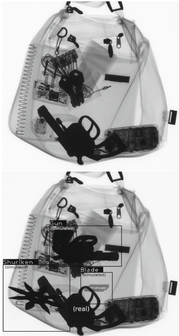
Fig. 8.23 Simulation of three threat objects onto an X-ray image of a backpack. The original X-ray image (Top) has only one handgun, whereas the simulated X-ray image (Bottom) contains the original handgun and the three superimposed three objects. The location of the bounding boxes can be easily defined because they correspond to the location where the foreground objects have been superimposed. [→ Example 8.4 ]
