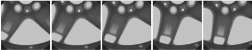
Fig. 2.3 Some X-ray images of an aluminum wheel (group Castings series C0001)
