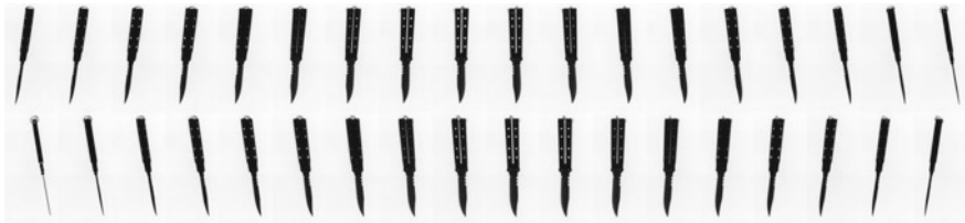
Fig. 2.10 A knife was rotated in 1^\circ and by each position, an X-ray image was captured. In this figure, X-ray images at 0^\circ, 10^\circ, 20^\circ, \dots, 350^\circ are illustrated (see series B00008 of group Baggage)
