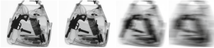
Fig. 4.34 Degradation of an X-ray image of 2208 \times 2688 pixels: Original image and degraded images with n = 32, 256, and 512 pixels
