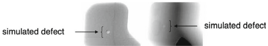
Fig. 8.8 Two generated defects using spherical cavities [1]
