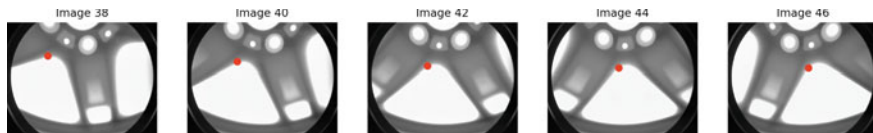
Fig. 3.10 Projection of a 3D point onto 5 different X-ray images of the same object in 5 different positions. [→ Example 3.5 🗺️]
