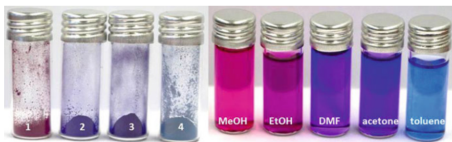
Fig. 21 Left: photography of compounds SP-Nitro@MOF-5 (1), SP-Nitro@MIL-68(In) (2), SP-Nitro@MIL-68(Ga) (3), and SP-Nitro@MIL-53(Al) (4) after irradiation with UV light ( \lambda = 365 nm, 1 min). Right: photography of SP-Nitro dissolved in solvents of varying polarity after irradiation with UV light ( \lambda = 365 nm, 1 min). Reprinted (adapted) with permission from Ref. [152]. Copyright 2017 American Chemical Society
