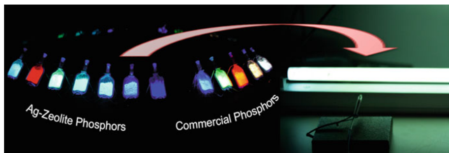
Fig. 6 Silver-zeolite-based phosphors and lanthanide-based commercial phosphors under 254 nm illumination (left). Working fluorescent lamp prototype using green-emitting silver-zeolite phosphor materials (right)
