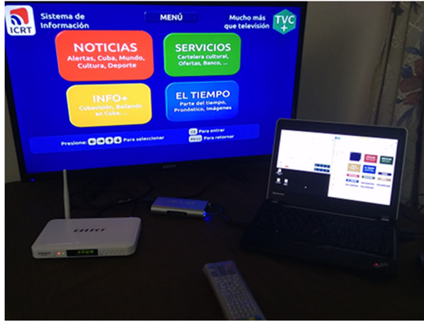
Fig. 5. Test scenario where the modulator is shown (in the center) that transmits the signal generated on the PC and is finally displayed on the TV from the STB.
