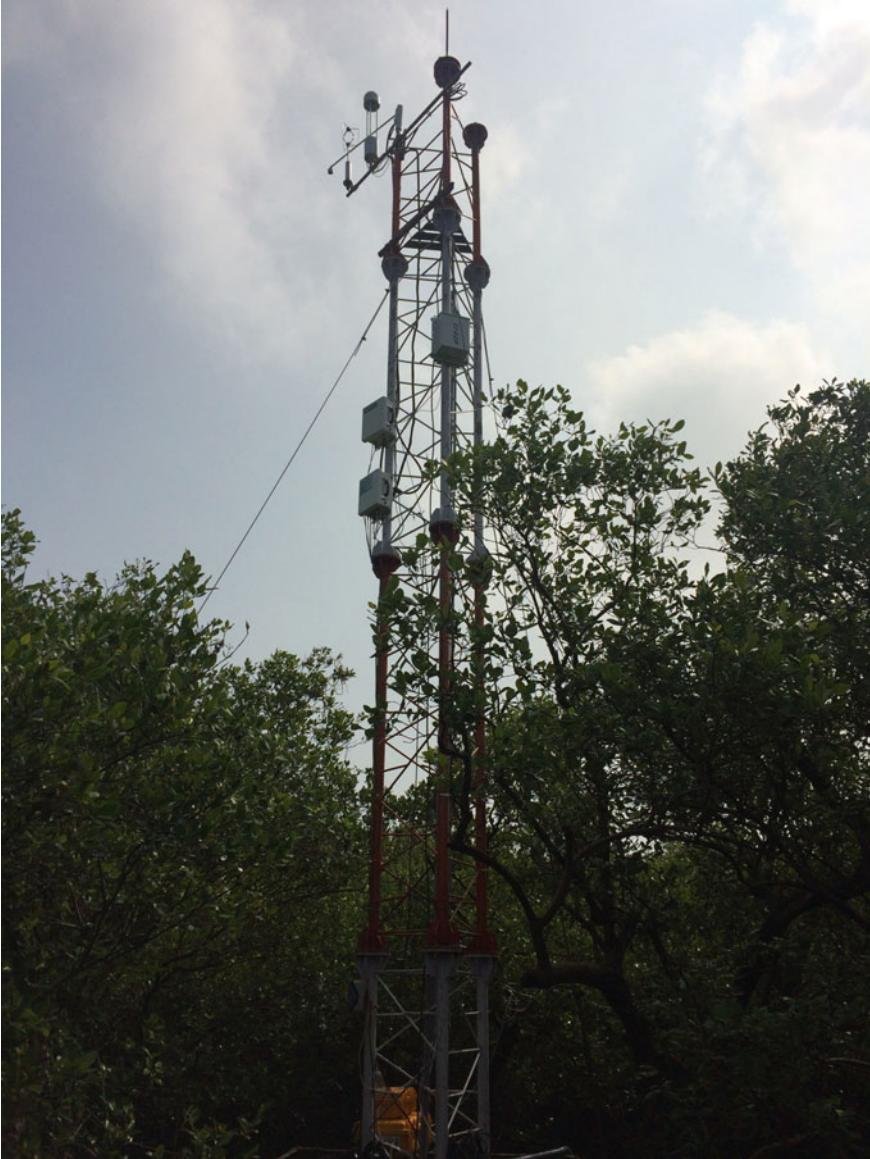
Fig. 2.1 A surface flux tower instrumented at multiple levels with eddy covariance and other associated measurement sensors at the Pichavaram mangroves, Tamil Nadu, India; this tower is part of the MetFlux India network
