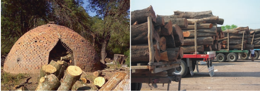
Fig. 8.6 Argentine half orange or beehive brick kiln, typical in Chaco for the production of charcoal (photo: Clelia Gomez). Prosopis alba trunks, harvested in the natural forest and on the way to a regional sawmill (photo: A. Verga)
