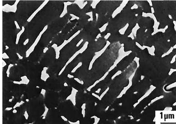
Fig. 2.8 Surface structure of Ti-29Nb-13Ta-4.6Zr alloy showing honeycomb pattern under the scanning electron microscope. [Reprinted with permission of Elsevier from Niinomi (2003)]
