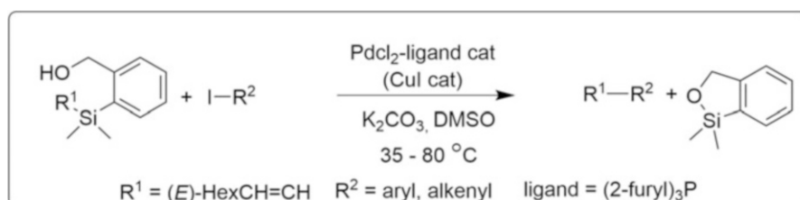
Scheme 9.6 Organosilicon-based cross-coupling of aryl and alkenyl iodides (Nakao et al. 2005)
