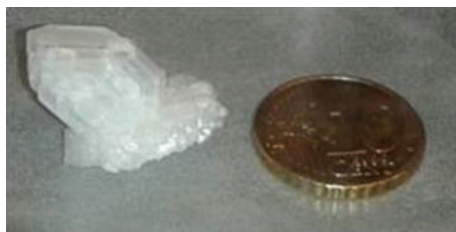
Fig. 13.4 Typical crystal aggregate of \text{Cs}_2[\text{Zn}(\text{NH}_2)_4] together with a 10 €-ct. coin for size comparison. Photograph taken while sample was stored in inert gas. From T. M. M. Richter, N. S. A. Alt, E. Schlücker, R. Niewa, Z. Anorg. Allg. Chem. Copyright 2016 by John Wiley & Sohns, Inc. Reprinted with permission of John Wiley & Sohns, Inc.
