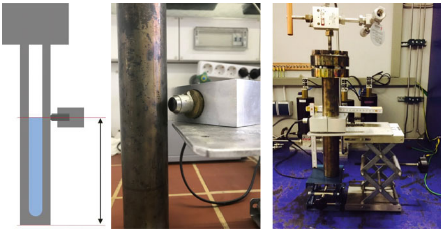
Fig. 7.3 Placement of the ultrasonic sensor and adjustment of the filling level
