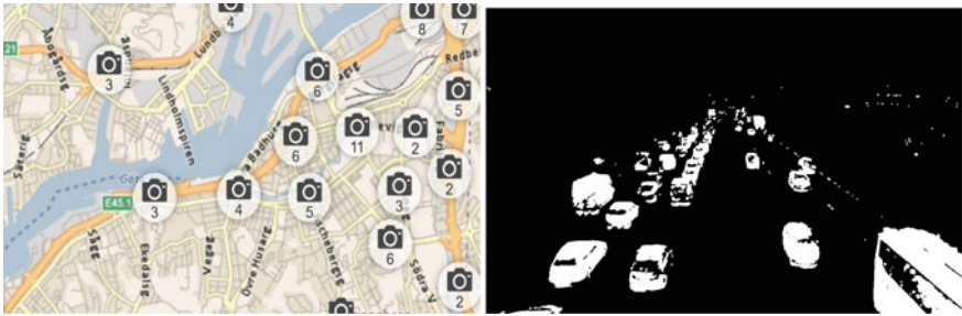
Fig. 2 (Left) Overview of a part of the traffic network and locations of (multiple) cameras where some of the images and data are collected from. Example from Goteborg downtown. Data provided by Trafikverket. (Right) Filtering one of the images for processing and counting (see Sect. 3 for details.)
