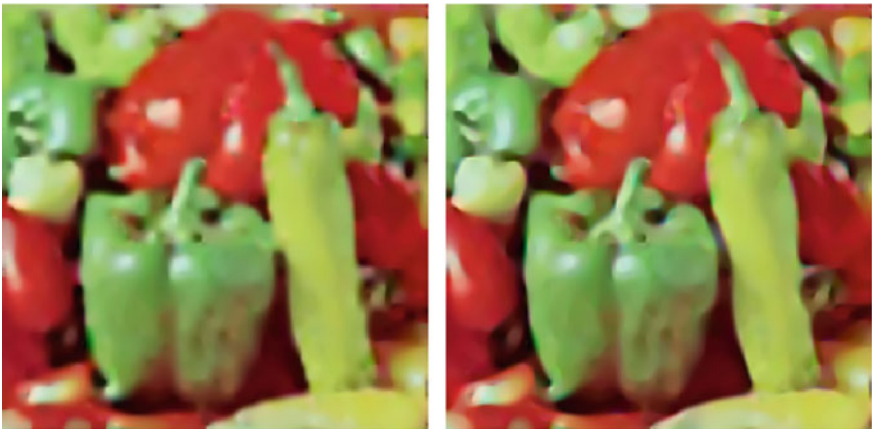
Fig. 6 RGB peppers image, reconstructed from randomly chosen 5% of pixel values using EED (left) or FOEED (right)
