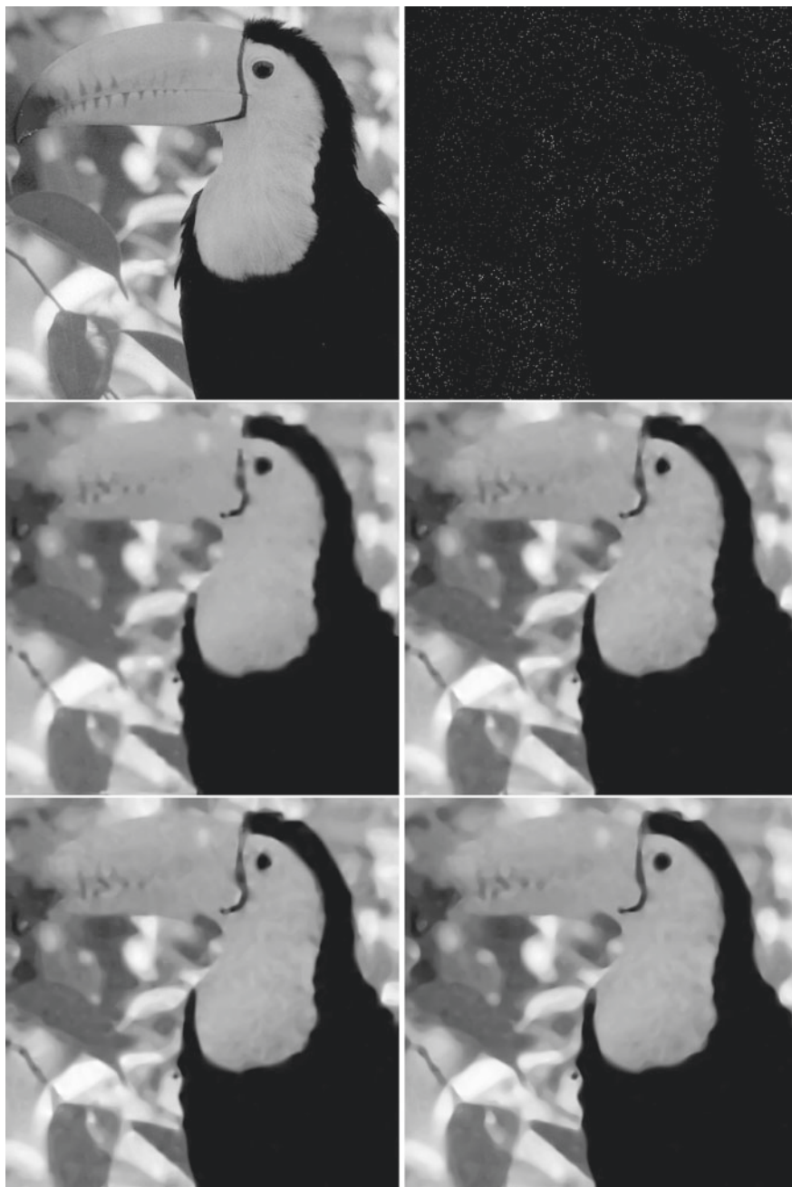
Fig. 2 1st row left: original toucan image of size 512 \times 512 ; right: randomly chosen 2% of pixel values; 2nd row left: EED based inpainted image; right: Li1 based inpainted image; 3rd row left: Li2 based inpainted image; right: FOEED based inpainted image
