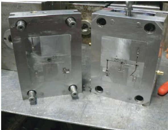
Fig. 20.2 A core/cavity mold set showing a central injection point and channeling to regions where five different parts are formed in one cycle
