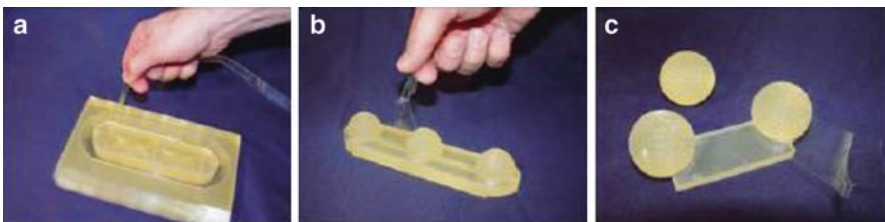
Fig. 9.2 Support material removal for three golf balls made using a Solidimension machine, showing (a) the balls still encased in a central region, being separated from the larger block of bonded material; (b) the support material is glued in an accordion-like manner so that the excess material can be pulled out easily as a continuous piece; and (c) the balls after complete removal of excess support material. (Photo courtesy of 3D Systems)
