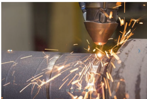
Fig. 10.11 Cladding on shaft. (Photo courtesy of Hardchrome Engineering) [20]
