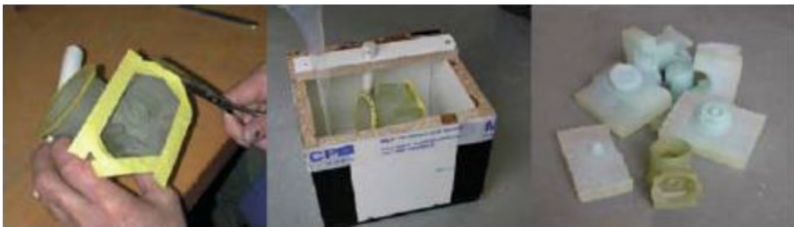
Fig. 16.21 RTV molding process steps. (Photo courtesy of MTT Technologies Group)
