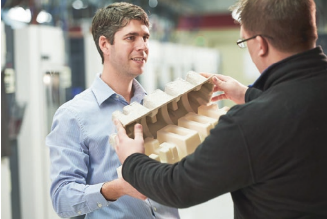
Fig. 20.7 A paper pulp molding tool shown with a molded packaging component. (Photo courtesy of RedEye Redeyeondemand.com )
