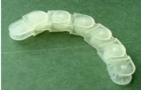
Fig. 19.5 Pulley-driven snakelike robot
