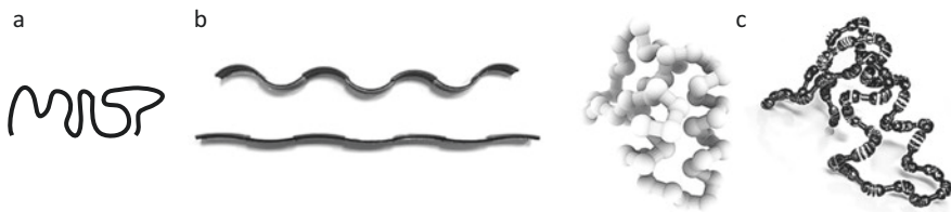
Fig. 19.19 Illustration of (a) 1D-to-2D shape-shifting by self-folding, (b) 1D-to-2D sinusoidal shape-shifting by self-bending, (c) 1D-to-3D strand by self-folding (Elsevier license number 4616800330874) [31, 33]
