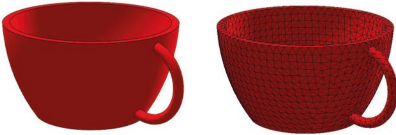
Fig. 2.2 A CAD model on the left converted into STL format on the right
