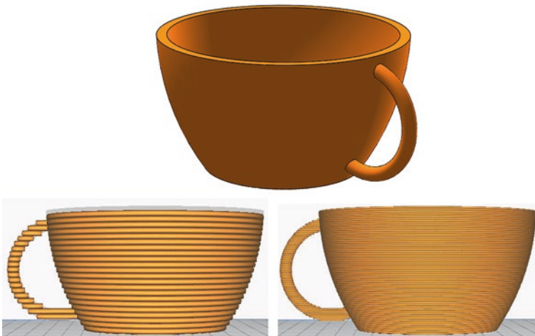
Fig. 1.1 CAD image of a teacup with further images showing the effects of building using different layer thicknesses
