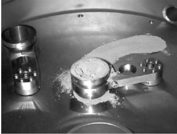
Fig. 5.15 3D-Micromac Powder Feed System. In this picture, only one of the powder feeders (located over the build cylinder) is filled with powder. (Photo courtesy of Laserinstitut Mittelsachsen e.V)
