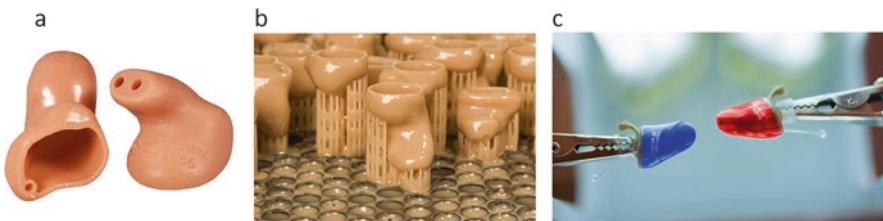
Fig. 2.11 RM of custom hearing aids, from a wax ear impression, on to the machine to the final product. (Photo courtesy of EnvisionTEC and Sonova) [47, 48]
