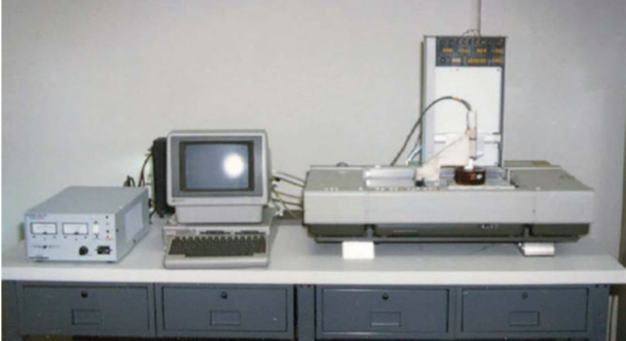
Fig. 2.8 The first AM technology from Hull, who founded 3D Systems (photo courtesy of 3D Systems)
