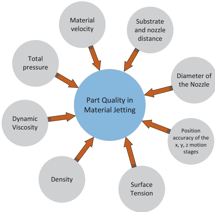
Fig. 7.16 Effective process parameters in MJT
