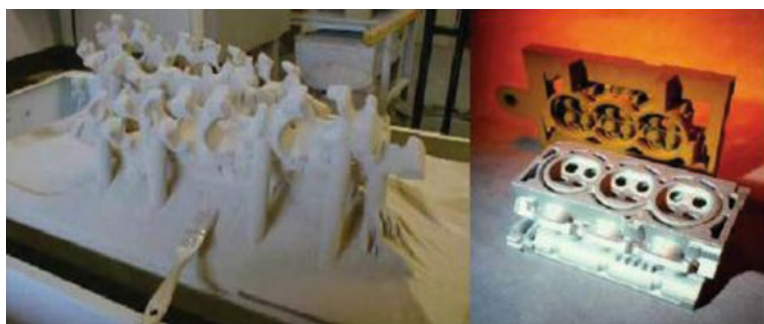
Fig. 16.20 Sand casting pattern for a cylinder head of a V6, 24-valve car engine (left) during loose powder removal and (right) pattern prepared for casting alongside a finished casting. (Joint project between CAD/CAM Becker GmbH and VAW Südalumin GmbH, made on an EOSINT S laser-sintering machine, photo courtesy of EOS)
