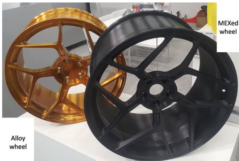
Fig. 6.6 Machined alloy (gold) and polymer MEX (black) 20 inch wheel by 6Sixty Design
