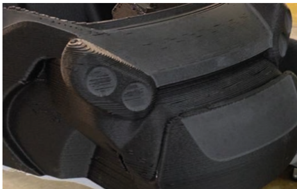
Fig. 6.8 Strati car front-end fabricated on a BAAM machine
