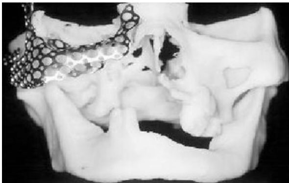
Fig. 21.3 Titanium mesh formed around a maxillofacial model
