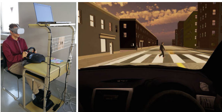
Fig. 58.1 Left: picture of the VR driving simulator including headset, steering wheel, pedals and the PC used to transfer data between them. Total cost of the whole equipment was below 500 $. Right: screenshot of the scenario represented in VR; a pedestrian is seen crossing the road from inside the car
