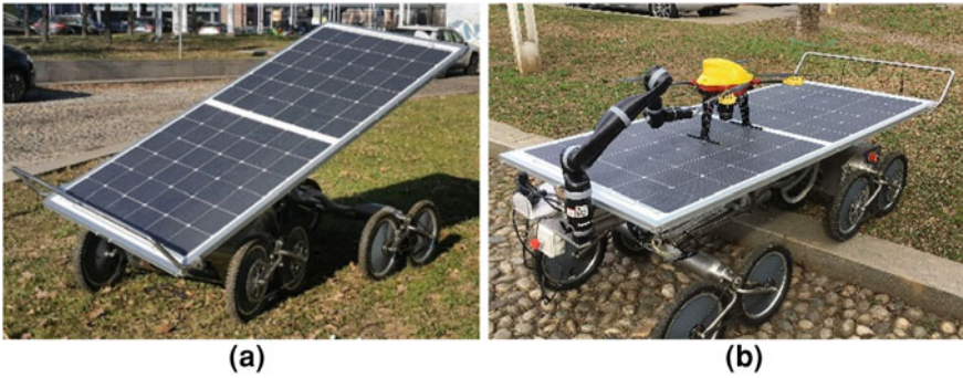
Fig. 6.2 Usage of the orientable upper panel during solar recharge (a) and for safe drone landing (b)
