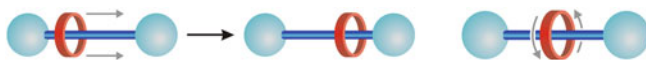
Fig. 21.1 Schematic representation of the translational (left) and rotational (right) movement of the ring in the case of rotaxanes (adapted after [3])
