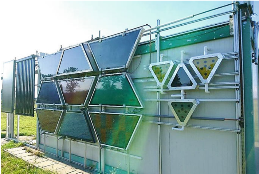
Fig. 1.5 Outdoor testing rig for the solar-thermal collectors in the R&D Institute of the Transilvania University of Brasov
