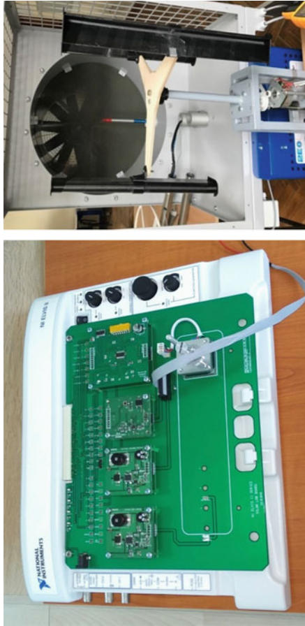
Fig. 14.4 NI Elvis II system with the RELab add-on (left); the scoop bladed wind turbine and the wind tunnel (right)
