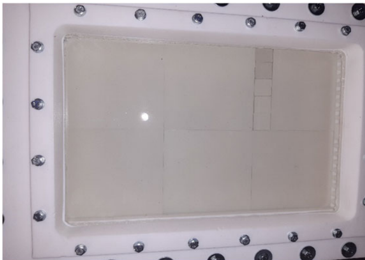
Fig. 24.1 The demonstrator photocatalytic reactor (before use)
