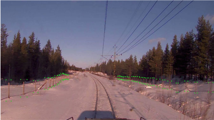
Fig. 26.1 Rectangular bounding boxes drawn around each visible reindeer fence pole
