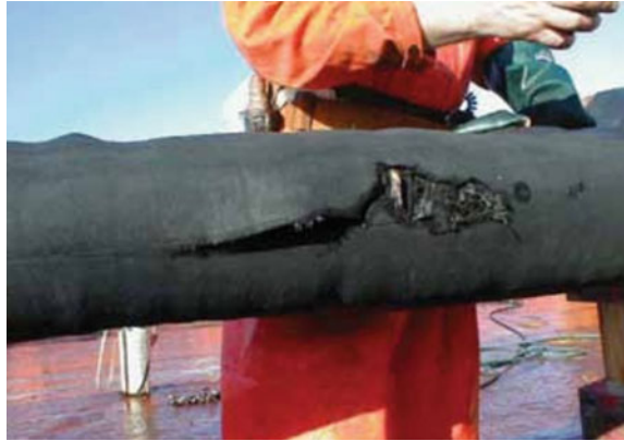
Fig. 5.5 Burst hose as a result of excessive pressure from pumping highly viscous oil [31]
