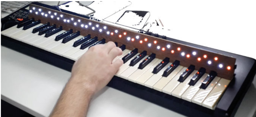
Fig. 6 The Illuminating Keyboard. The plywood structure holding the LED array docked to the MIDI keyboard controller
