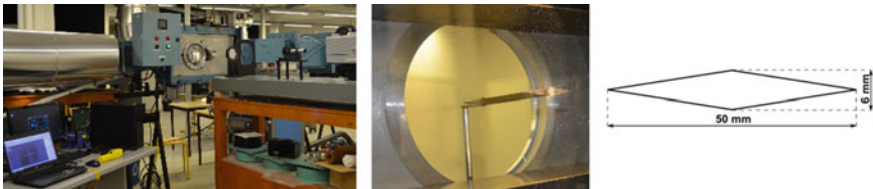
Fig. 3 (Left) Global view of the wind tunnel and Schlieren test bench and a detailed view of the wind tunnel model of the aileron in the test section, (right) schematic view and dimensions of the wind tunnel aileron
