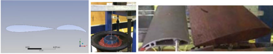
Fig. 4 Wind tunnel models. Main wing NACA 0015, chord c = 125 mm, span b = 300 mm. Flap EPPLER 561 17% thick, chord c_f = 65 mm, span = 300. Reduced frequency k is based on c
