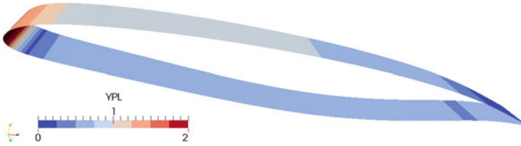
Fig. 5 Contours of the cell height y^+
