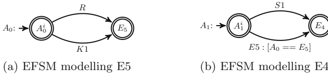
Fig. 3. EFSMs for intermediate failure events, E4 and E5 of the fault tree
