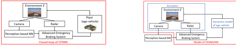
Fig. 9. Closed-loop system, S_2 , of the CPSNN considered for the case study of the modular pattern (left) and the corresponding model of its CPSNN/NN composed with the perception-based NN in the system (right)
