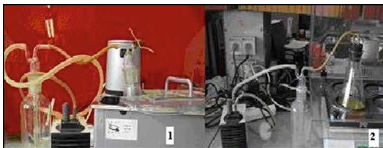
Fig. 4.1 Simple system for analysis of microbial VOCs. To increase stability and sensitivity of the method, the flask with the sample has been placed to thermostat at 30 °C (1), and for continuous analysis of VOCs during cultivation, the flask with the sample has been placed to the shaker (2)
