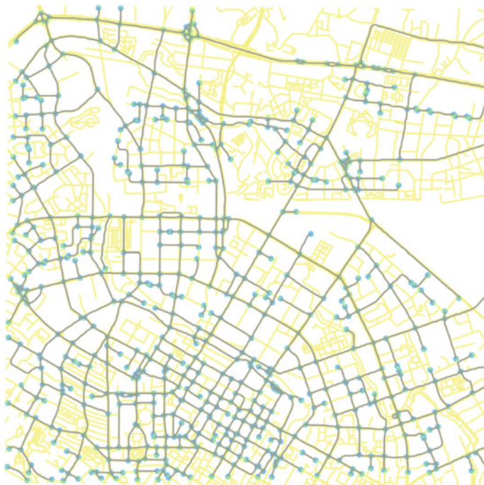
Fig. 11.10 The extracted road graph with ground-truth reference graph (yellow)
