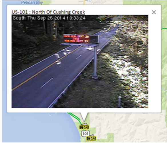
Fig. 13.5 Caltrans District 1 CCTV image to confirm CMS message
