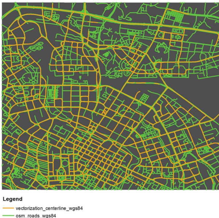
Fig. 11.9 A visual comparison of the extracted road network and the OSM road reference layer
