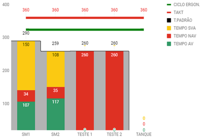
Fig. 7. Yamazumi board after, with the improvement of the new device.
