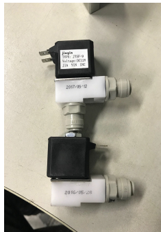
Fig. 2. Solenoid valve used in the model A, every gap is a possible leak point. Source: Authors
