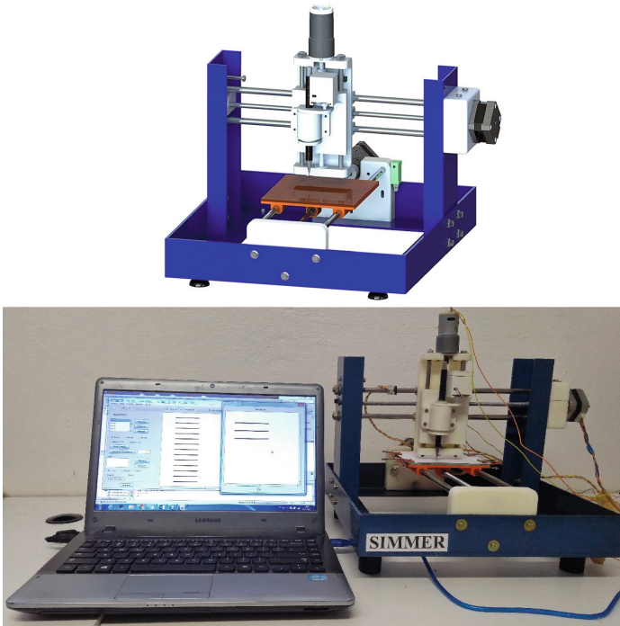
Fig. 2. Machine final design and its prototype. Source: Elaborated by authors.
