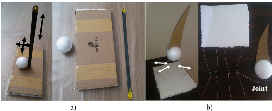
Fig. 2. a) The physical model of a Band Saw and b) the physical model of the Spine of the European Hedgehog [31].
