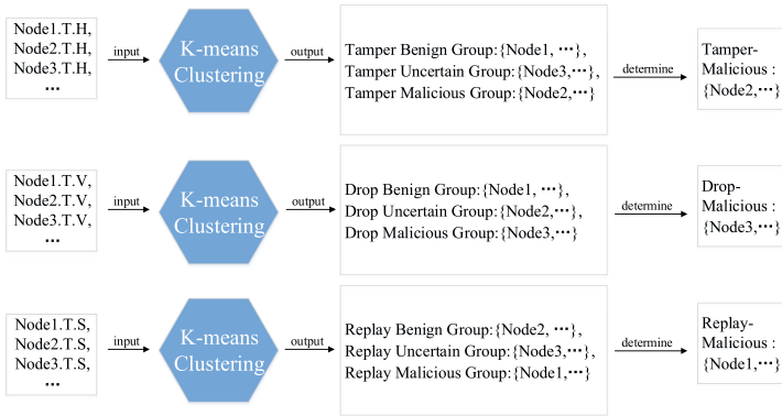
Fig. 3. K-means based malicious node detection
