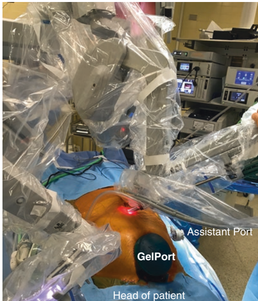
Fig. 22.8 Robotic-Assisted Pancreas Transplant surgical positioning: The assistant surgeon positions himself to right side of the patient near the head of the bed. The robot is docked on the left side of the bed. The lead surgeon is controlling the robot from the console. The scrub nurse and surgical table on the right side of the patient
