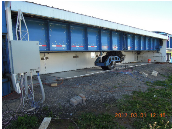
Fig. 1. a) Comparison of slab mean temperature and ELTD between uncovered concrete section (Outdoors series) and section under the HVS shed (Test section series), b) tested section, environmental chamber is open on its north side
