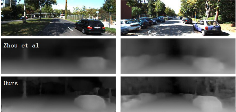
Fig. 1. Example predictions by our method on KITTI dataset of [7]. Compared against [23], our approach recovers more details in the scene.
