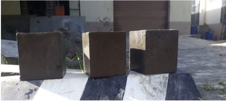
Fig. 6 Cubes for testing
