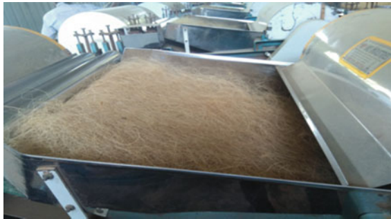
Fig. 3 Processed and combed coconut fibre
