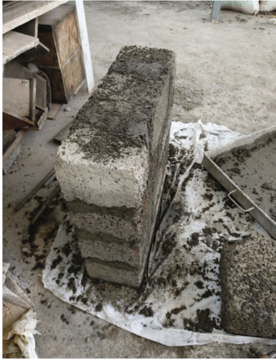
Fig. 2 Casting of concrete block masonry panel
