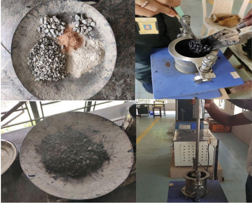
Fig. 4 Sampling, Mixing, Pouring and Compaction of Mix II
