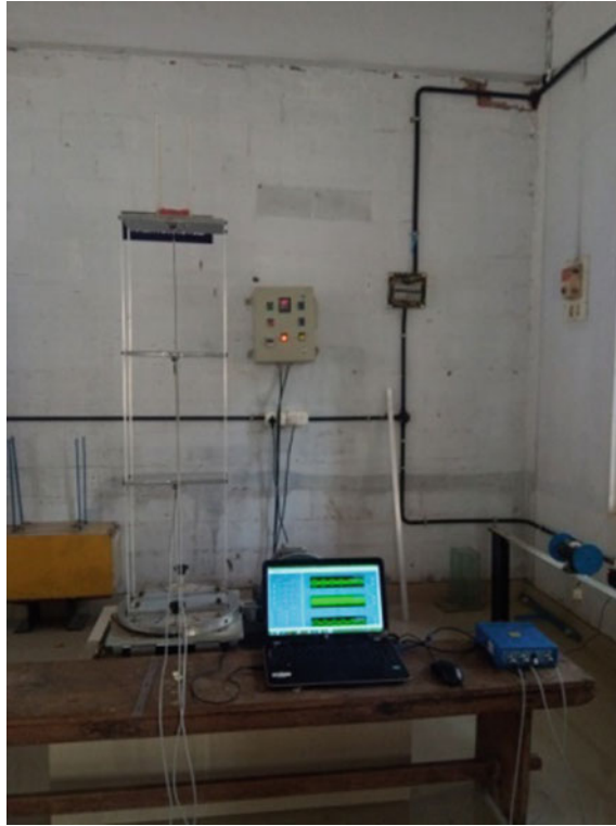
Fig. 3 Experimental setup with damper at third floor
