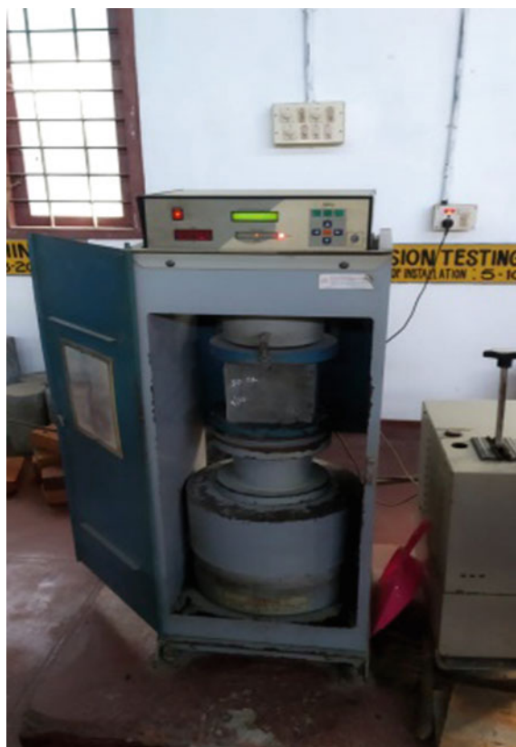
Fig. 1 Testing of compressive strength
