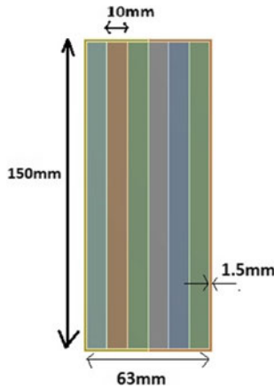
Fig. 4 Modeled view of GFRG laminated beam with aspect ratio 2.5 strengthened externally with CFS (C section)
