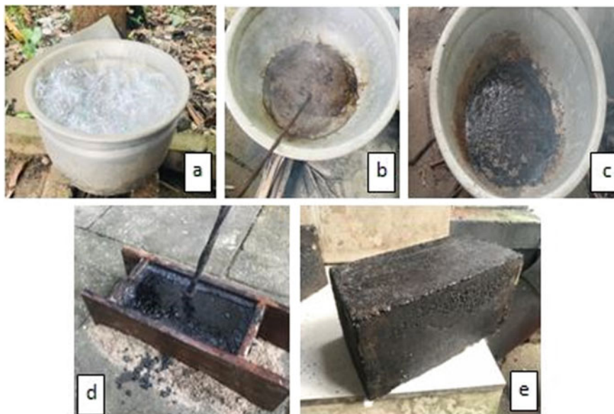
Fig. 1 a Cleaning and shredding of PET bottles. b Melting of plastic. c Addition and mixing of sand and bitumen. d Compaction of brick using steel rod. e Prepared brick
