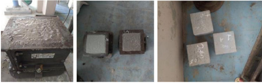
Fig. 3 Casting of cubes
