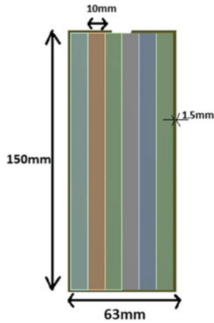
Fig. 5 Modeled view of GFRG laminated beam with aspect ratio 2.5 strengthened externally with CFS (U section)
