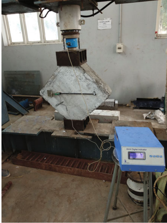
Fig. 3 Setup of in-plane diagonal loading
