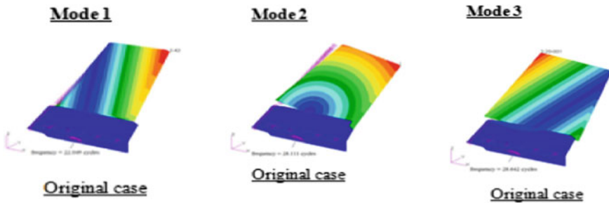
Fig. 5 Mode shape of original fin design
