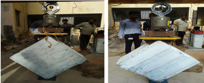
Fig. 7 Masonry Shear strength test
