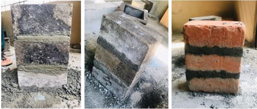
Fig. 2 Masonry prism of plastic-M-sand bricks, Plastic-Foundry sand bricks and normal burnt clay bricks
