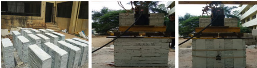
Fig. 6 Masonry bearing capacity test
