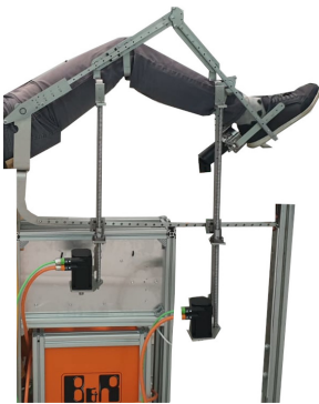
a) experimental model of the hip-knee rehabilitation module
