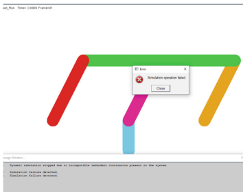
Fig. 18. Simulation failure detected by ADAMS
