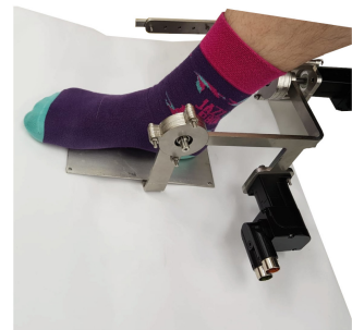
b) experimental model of the ankle rehabilitation module
