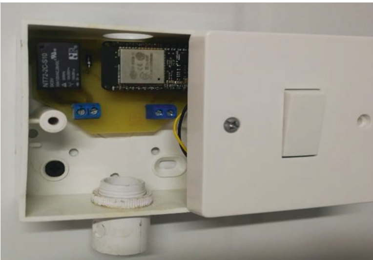
Fig. 3.22 Secured smart home switching system smart switch implementation
