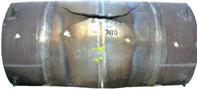
Fig. 5.4 Destroyed cylindrical shell
