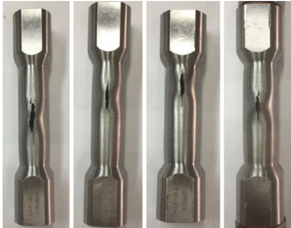
Fig. 5.1 Limiting strains depend on stress state factor \Pi
