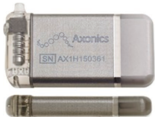
Fig. 10.2 The Axonics® rechargeable Sacral Neuromodulation (r-SNM®) system for the treatment of urinary and bowel dysfunction. (Reused with permission. Copyright John Wiley and Sons (24))
