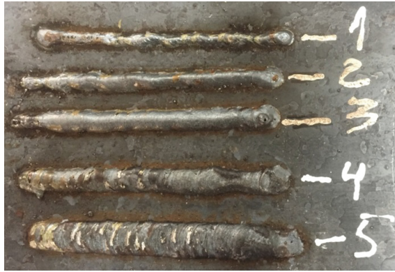
Fig. 2. Deposited beads using different process parameters.
