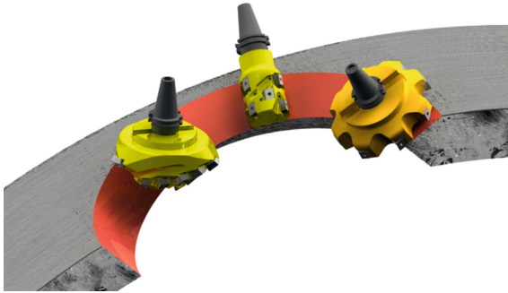
Fig. 2 Bevel shape-forming schemes with corner, cylindrical, and end mills
